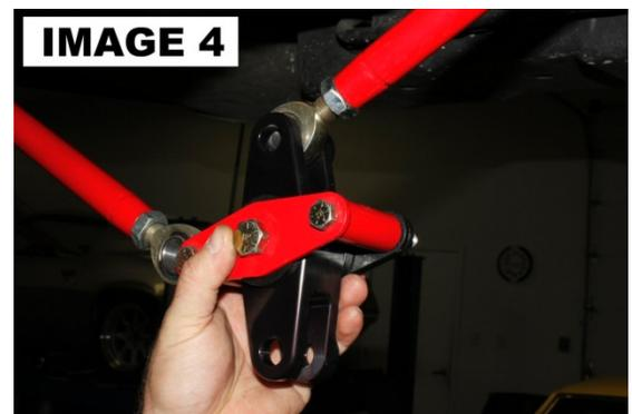
6. Connect the Watts linkages to the new pivot using the new provided 5/8" x 2" bolts, washers, and lock washers. **IMAGE 4**
