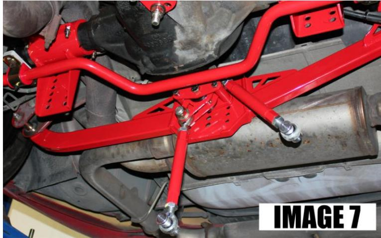
17. It is not necessary to torque this hardware. To prevent pre-load on the bushing, tighten the bolts until the pivot just begins to bind the bushing. As the bushings wear in, these bolts can be tightened further.
