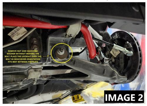
4. After you have selected the setting that best suits your application, remove the eccentric bolt and install the matching lockout for the other side of each mount and bolt it together
