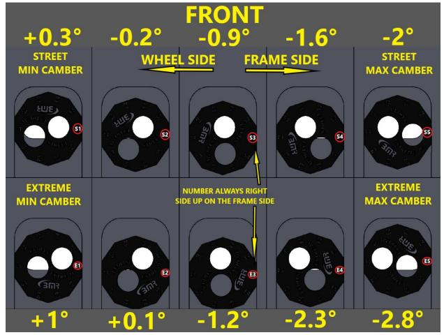
**NOTE**: If more or less camber is desired, use a different flat on the lockout to move the control arm **IN** for more positive camber or **OUT** for more negative camber (see table) Caster can also be adjusted by staggering the lockouts on the lower control arm. If more fine adjustments are needed, use BMR part number **WAK561**
