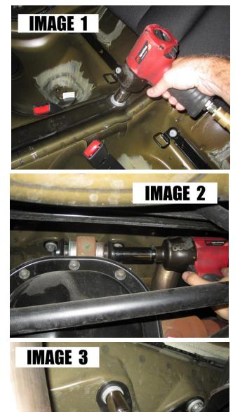
10. Re-install the assembly into the car and insert the rear upper mounting bolts. Tighten to 85 ft/lbs.
