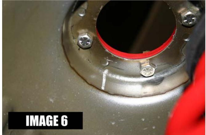
5. Remove the brace and de-burr the mounting holes.
