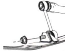
6. Using a 15mm socket, remove the (4) bolts on the upper shock mount. See **IMAGE 2** for reference.
