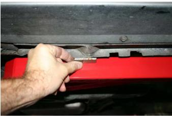
BMR Subframe connectors ship with additional reinforcement plates that may be welded in if desired. They are designed to join the factory pinch welds on the rocker panels to the Subframe Connectors. The reinforcement plates are not necessary for light duty street applications but are recommended for aggressive road racing, high horsepower drag racing applications or when using the BMR Trak Pak or Xtreme Duty torque arms with weld-in cross-member. See image below for installation example.
