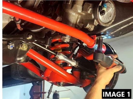
3. Remove the four (4) bolts holding the rear sway bar saddles on the frame with a 1/2" socket. **IMAGE 1**
