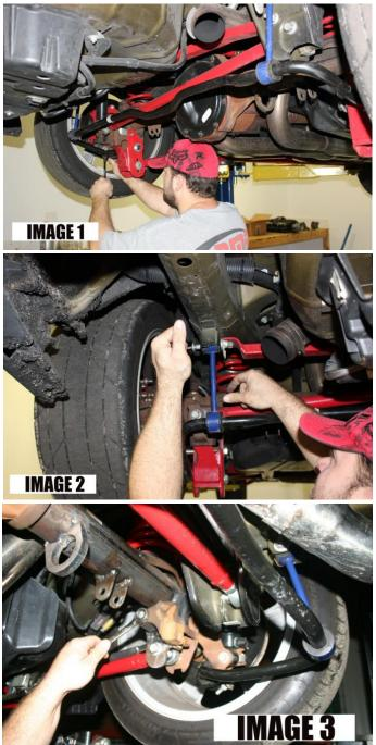
7. Directly above the control arm bolt is the axle damper weight that must also be removed for this installation. Remove it using a **15mm** socket or wrench as shown in **IMAGE 3**.
