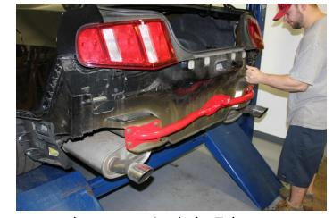
9. Measure from the ground up to the center parachute mounting hole. Take a measurement from the center of this hole.
