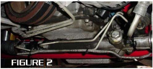
31. Bend the ends of the brake lines in such a way that the mounting brackets line up with the brake line mounting tabs on the k-member. You may also have to cut the brackets and re-bend them in order to fit properly. Insert bolts and tighten. Once connected, brake lines should look similar to figure 3 below.
