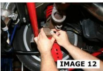
14. As in step #5, install the gold spacer and 14mm x 110mm bolt and nut into the OE control arm mounting hole and leave the bolt loose. See **IMAGE 13**.
