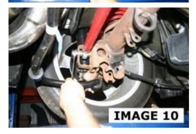
12. Slide the BMR Drivers' side relocation bracket up onto the mount. The rear leg of the mount should fit up into the OE bracket of the rearend on the backside of the Panhard rod mount. Insert the provided spacer behind the upper hole as shown in **IMAGE 11**.
