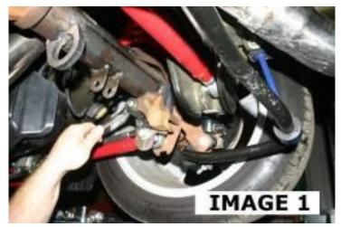
3. Using an 18mm socket or wrench, remove the lower control arm bolt as shown in **IMAGE 2**. Lower control arm to gain access to mount area.
