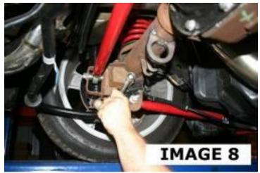
10. Using the 18mm wrench, loosen the control arm mounting bolt and lower the control arm out of the way. See **IMAGE 9**.
