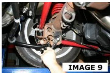
11. Using an 18mm wrench, remove the Panhard rod bolt as shown in **IMAGE 10**.
