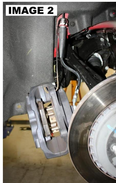
3. Using a 15mm socket, remove the brake caliper bolts. Remove the calipers from the brake rotors and hang them in the wheel-well using a piece of wire. (**IMAGE 2**)
