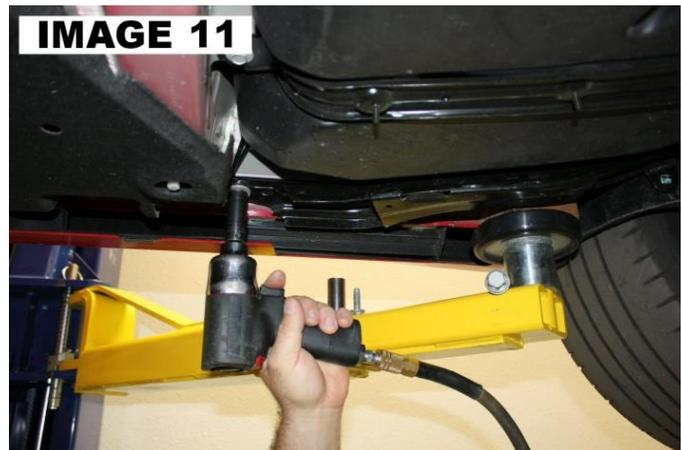
13. Move to the rear of the cradle and do the same. Use a 15mm socket to remove the cradle braces (one per side) and then the 18mm socket to remove the main rear cradle bolts.
