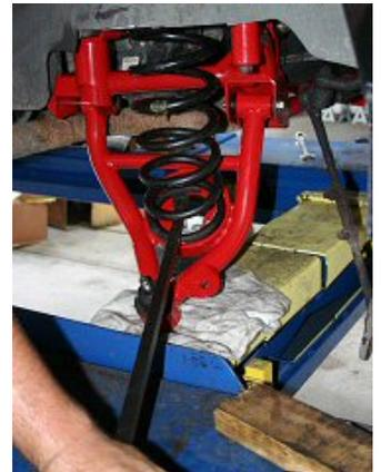
13. Once the spring is seated properly in the cup, carefully lift the A-arm until the ball joint seats into the spindle. Install the castle nut and tighten. Insert a new cotter pin.
