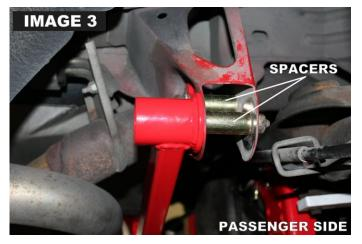
cross-member. Torque the smaller driver's side bolts to 47 ft/lbs. and the passenger side bolts to 83 ft/lbs.
