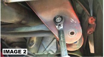
interference, you may need to lift or lower the rear end in order to get the bolt all the way out. (IMAGE 2)
