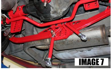
bolts until the pivot just begins to bind the bushing. As the bushings wear in, these bolts can be tightened further.
