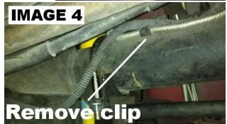
**NOTE:** In order to mount the brackets to the rear end, it is necessary to bend the brake lines up out of the way. Once the installation is complete, the lines can be re-positioned over the axle clamps.
