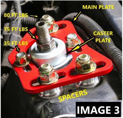
height down. These spacers may need to be removed if the vehicle has been lowered to prevent bottoming out.
