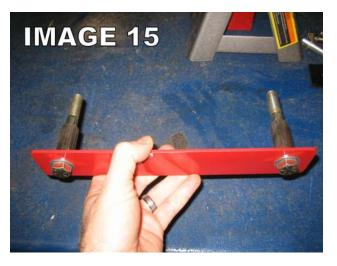
30. Proceed to the driver's side. The driver's side frame rail has a frame reinforcement that makes it differ from the passenger side. This requires a different reinforcement plate. Position the plate as shown in **Image 15b** and duplicate steps 24-29 using the remaining spacers and same length bolts.
