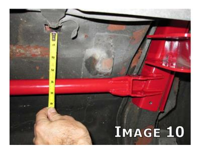
the reading from each strap mount relief is equal and falls within the range listed above.
