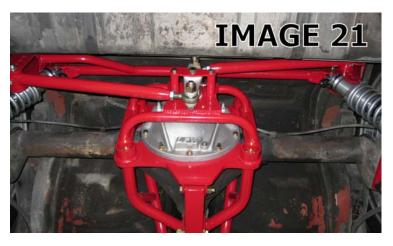
over the exposed thread and tighten to 80 ft/lbs. *NOTE:* the Watts link pivot should be vertical (straight up and down) with the suspension loaded. It may be necessary to adjust the rod end in order to achieve this.
