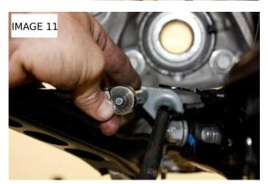
13. Using the 18mm socket and wrench, remove the lower trailing arm as shown in **IMAGE 12**.
