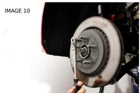
12. Using the 10mm socket, remove the emergency brake cable from the spindle as shown in **IMAGE 11**.
