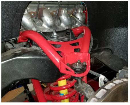
pops loose. NOTE: A pickle fork may also be used to loosen the ball joint.
