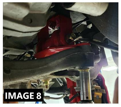
15. Reclip the brake line, abs sensor, brake hose, wiring harness and ride height sensor
